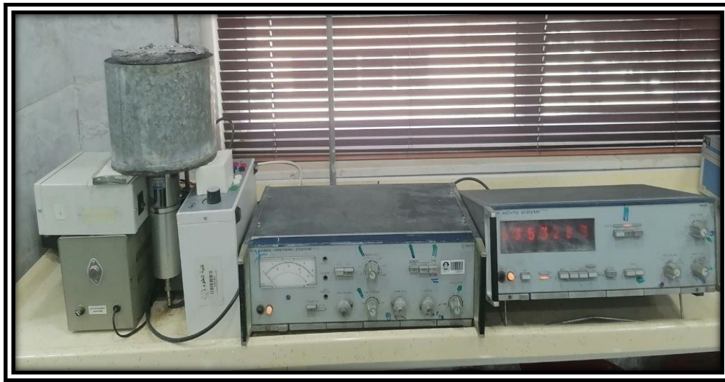
Fig. 3: Soil erosion measurement system using Cesium-137 (Cs-137)
